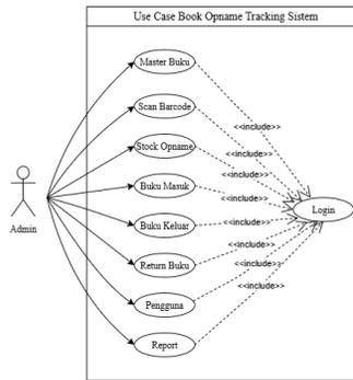
**Gambar 3.** Use Case Diagram
