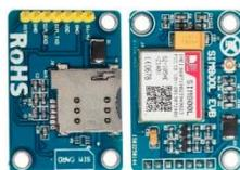
**Gambar 8. Modul GSM SIM800L**
