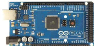
**Gambar 7. Arduino Mega 2560**
