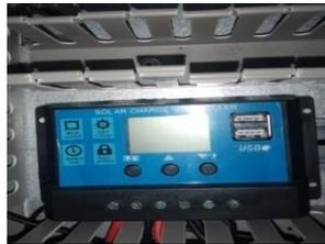
**Gambar 2. Solar Charge Controller**
